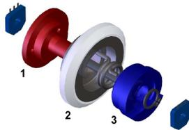
Fig. 5: Assembly drawing of spring mounted in wheel
